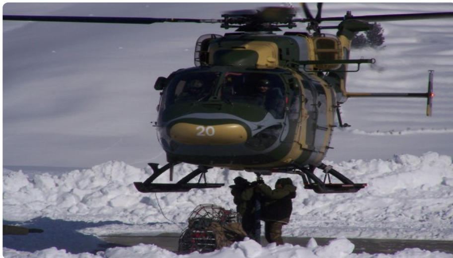
Underslung load on the indigenous Advanced Light Helicopter (ALH)
