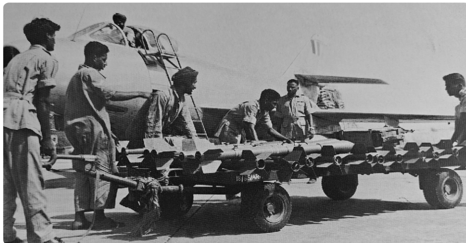
Mysteres being armed with T-10 air to ground rocket projectiles
