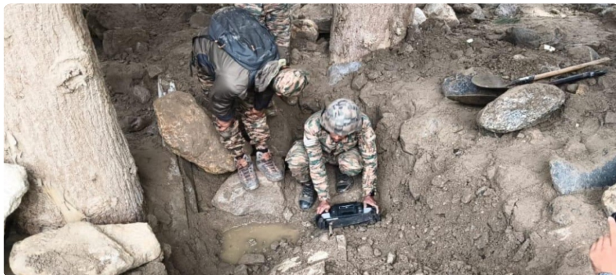
Indian Army troops using a Ground Penetrating Radar to detect missing persons under debris (Photo tagtv.info)
