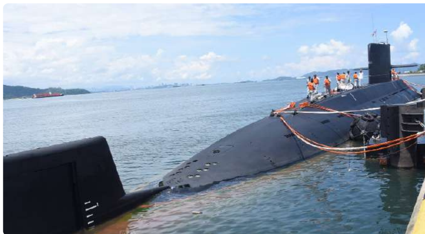
Aft Casing of PNS Hangor showing Active Sonar Decoy Dispensors (photo courtesy Royal Malaysian Navy)
