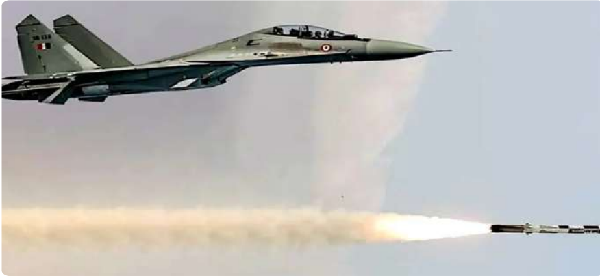
Indian Air Force Su-30 MKI firing BrahMos air to surface missile (Photo ANI)
