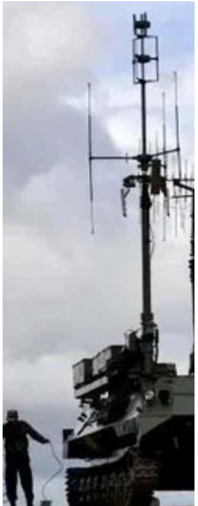
A Russian army Pole-21 jamming system in Ukraine (Russian state media photo)
