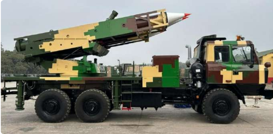
Suryastra MLRS with cone-shaped mock-ups mounted on the missile transport-launch containers (Open source photo)
