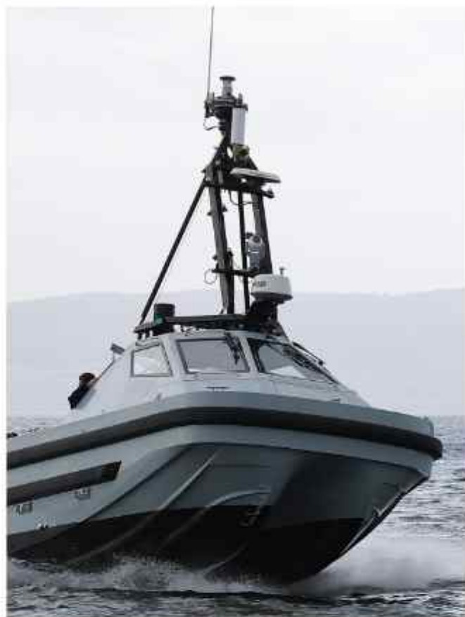
The future of mine hunting - RNMB Harrier, an Autonomous Mine Counter Measures vessel, part of a recently formed Maritime Autonomous Systems team in UK Navy (photo by L.Phot Stevie Burke, credit commons.wikimedia.org)
